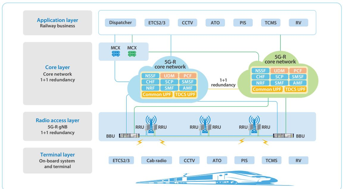
Fig. 1. ZTE FRMCS network architecture.
